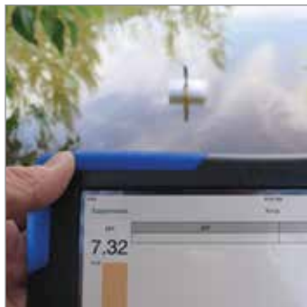
With the sensor raft floating 4 m from shore, data were recorded on an iPad using the Graphical Analysis app
