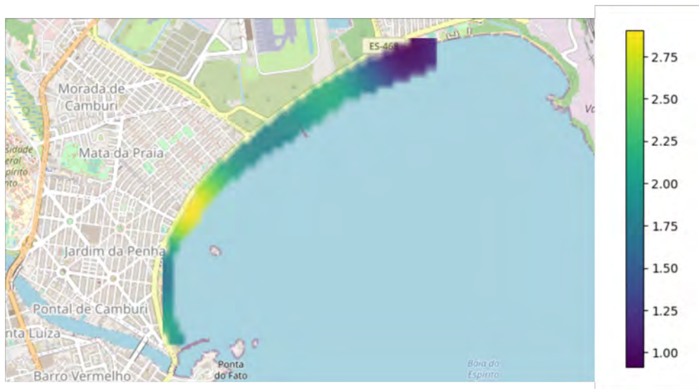
Figure 6: GP prediction of the radiation dosage field overlaid onto the geographical boundaries of Camburi Beach
